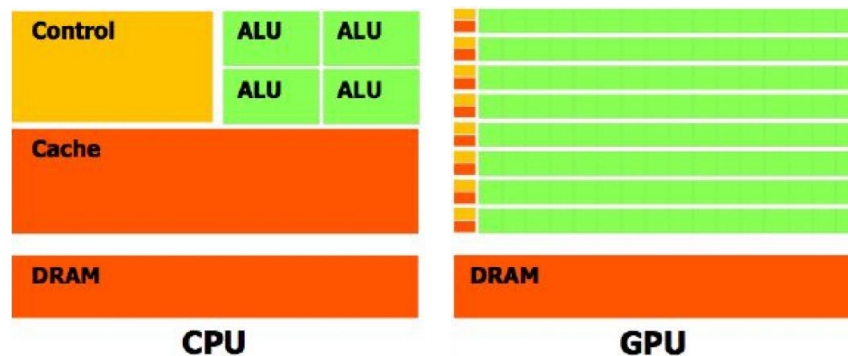
Figure 2.2: Internal components of processing units - CPU and GPU
